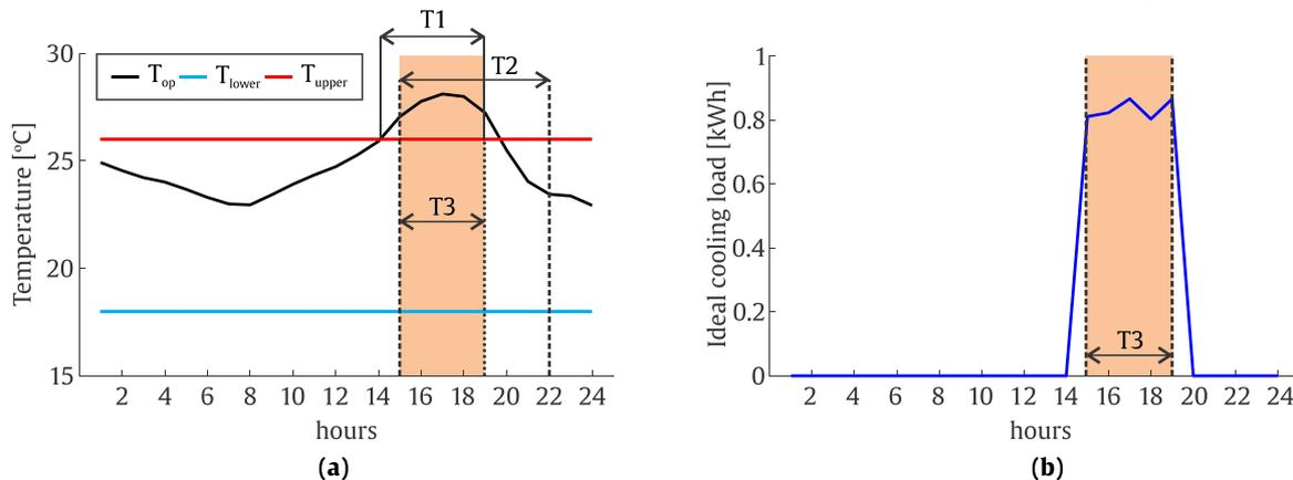
Fig. 12. Example of simplified methodology to evaluate the hybrid operation mode in residential buildings. T1 = period out of range, T2 = occupied period, T3 = occupied period out of range. The results are for the living room of the case study during March 28 in Porto Alegre (WMO = 839710). (a) Temperatures of the naturally ventilated model; (b) Period to sum the thermal ideal loads for cooling.
