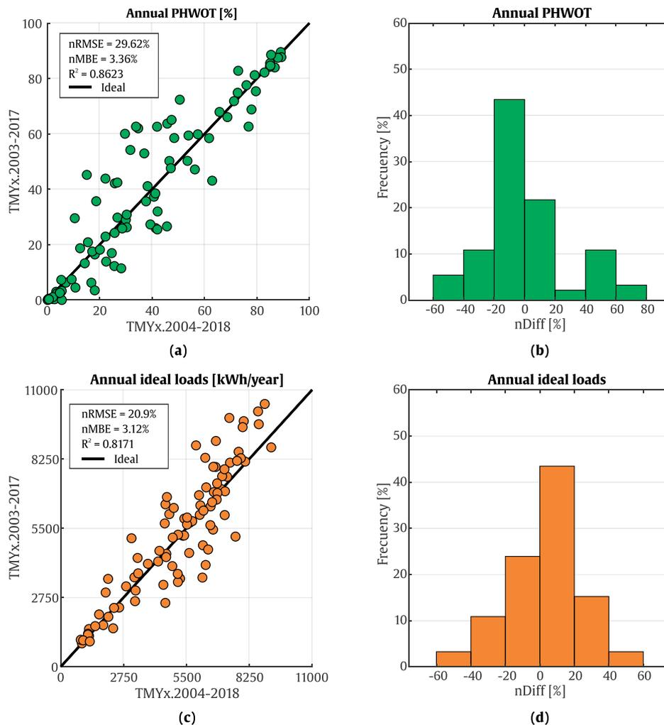
Fig. 16. Comparison of annual BPS results for the target residential building obtained by both databases TMYx.2003–20017 and TMYx.2004–2018 in 92 Brazilian locations.
