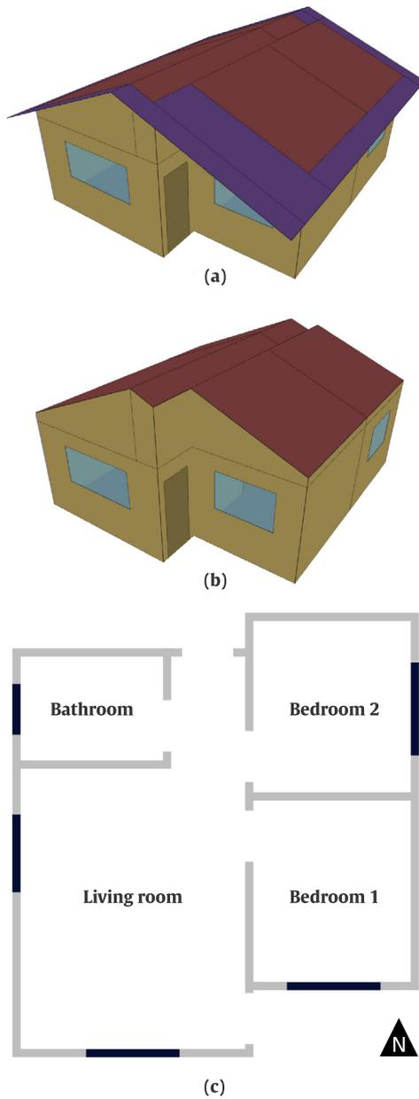
Fig. 11. Residential building models used in comfort and thermal load simulations: (a) target building; (b) reference model; (c) floor-plan view.
