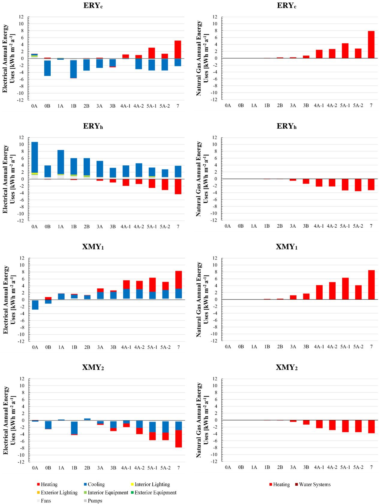
Figure 4: Deviation of final energy uses simulated with extreme years with respect to TMY<sub>x</sub> simulations: annual electrical energy uses (on the left) and annual natural gas uses (on the right).
