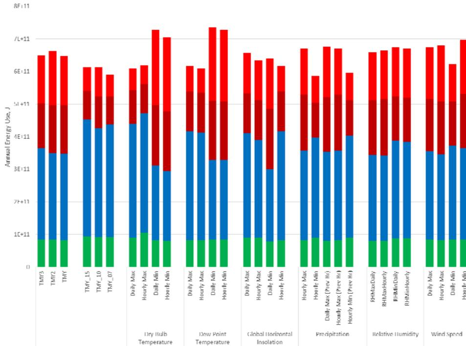
Figure 3. Heating, Cooling and Fan Energy Use for Initial Set of XMY and TMY for Medium Office, Washington Dulles
